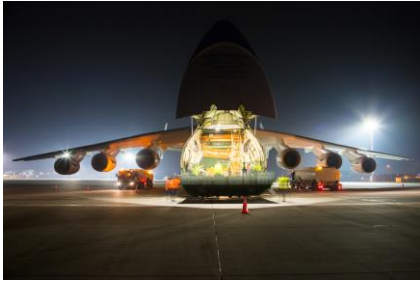
Caption: With a wingspan of 88.4 meters, a length of 84 meters and an empty weight of 285 tons, the six-engine Antonov An-225 is the longest and heaviest cargo aircraft in the world. Here: The unloading of the Antonov An-225 at Rzeszów Airport in Poland. (Quelle: Gebrüder Weiss / Damian Szymula)
